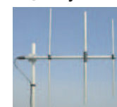
WY108-3N Airband 3 element Beam • Freq: 108-137MHz • Gain: 7 dBi • Boom: 1.4m
